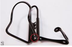
Using a 12mm bolt, nut and washer, bolt the bottom of your bottle cage to the tab on the longest side of the bottle cage riser. Tighten the bolts so that the cage can rotate under pressure but not freely.
