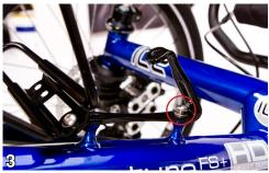
Using a 16mm bolt and washer connect the riser mount to the cruciform with the tabs facing forwards & down. Leave this bolt slighty loose.
