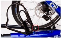
Using the other 16mm bolt and washer fix the riser mount to the cruciform and tighten both 16mm bolts.
