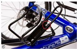
Finally rotate the bottle cage and connect it to the second tab using the 12mm bolt and 2 washers.
