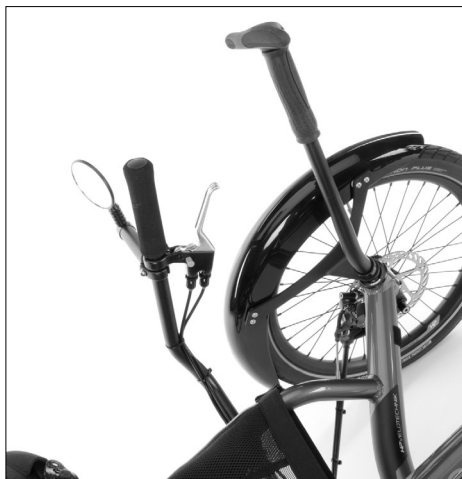
Standing-up aid mounted on a Gekko fxs.
